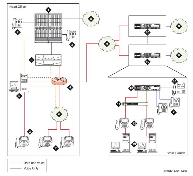
Figure 12: Sample configuration of the IG550 in a Communication Manager network
